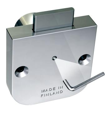
All **ABLOY**<sup>®</sup> cabinet locks are delivered with a default action where key is removable only in locked position. By adjusting the hexagonal bolt on the rear reverse of the lock key can be removed both locked and unlocked positions.
