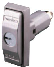
Medeco's high security T-handle inserts provide most of the same vandal resistant features of the complete Medeco T-handle in an economical retrofit package. 300 Series stainless steel components and drill shields, defy drills, chisels, punches and other common vandal attacks. The lock cylinder loads behind the handle and is protected from drilling and pulling by a free-spinning hardened steel cover.
